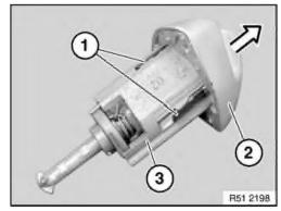
Remove catches (1) and detach cover (2) from lock cylinder (3).
